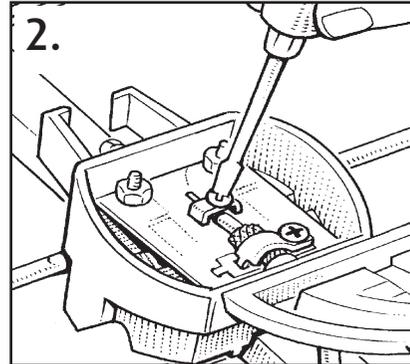
Loosen the screws on the 2 terminals in the Dipole. Feed the inner core to one of the terminals and the twisted braid into the other. Tighten screws and close Dipole Cap.
