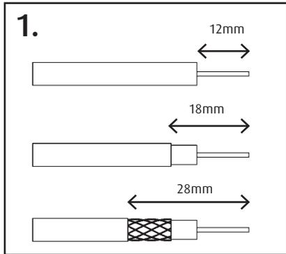
Using a sharp knife prepare the Coaxial Cable as shown.
